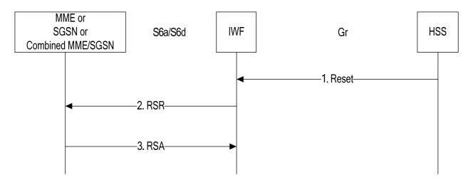
Figure 7.7.1-1: Mapping of Reset Procedure for scenario with one IWF
