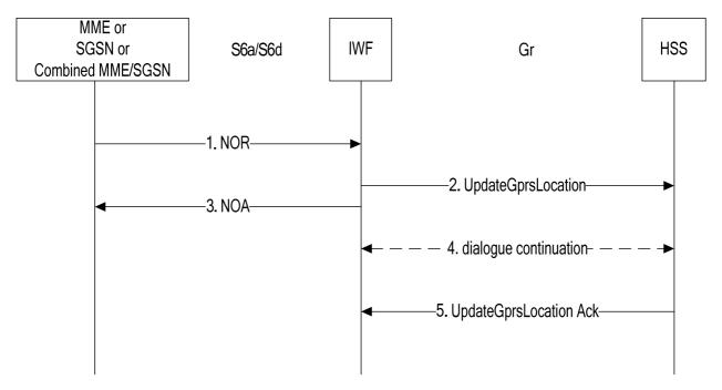
Figure 7.8.1-1: Mapping of Notification Procedure for scenario with one IWF
