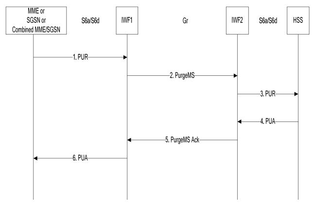
Figure 7.4.2-1: Mapping of Purge Procedure for scenario with two IWFs
