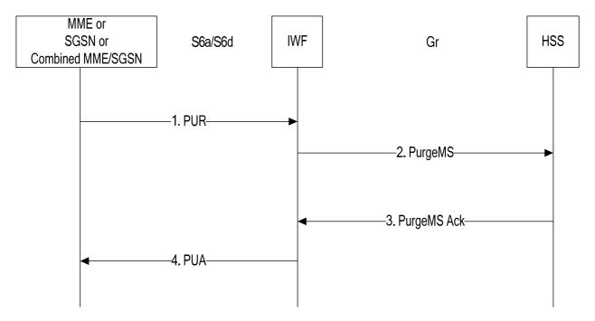
Figure 7.4.1-1: Mapping of Purge Procedure for scenario with one IWF
