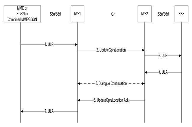
Figure 7.2.2-1: Mapping of Update Location Procedure for scenario with two IWFs
