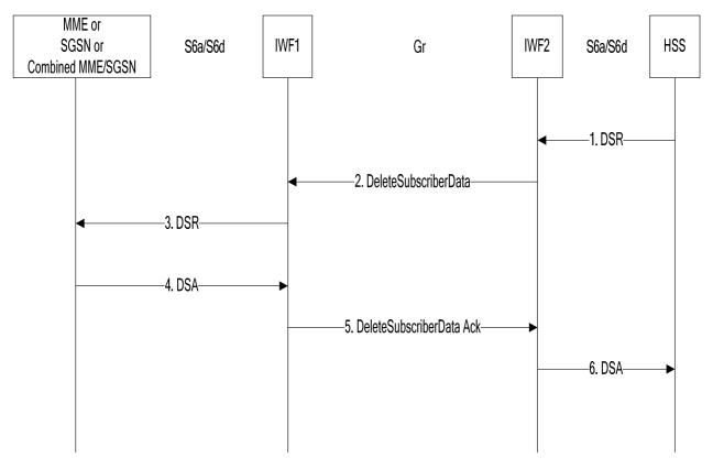
Figure 7.6.2-1: Mapping of Delete Subscriber Data Procedure for scenario with two IWFs
