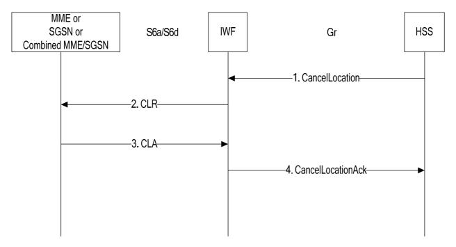
Figure 7.3.1-1: Mapping of Cancel Location Procedure for scenario with one IWF
