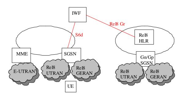
Figure 4.3.2-2 IWF Scenario two network deployment: visited EPS with E-UTRAN and UTRAN/GERAN, home Rel8 UMTS/GPRS only
