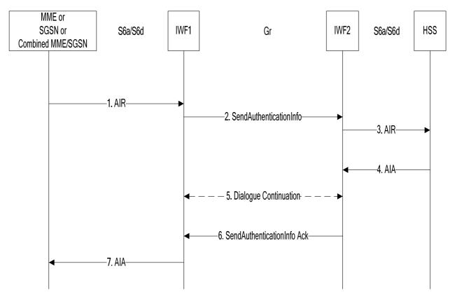
Figure 7.1.2-1: Mapping of Authentication Info Retrieval Procedure for scenario with two IWFs
