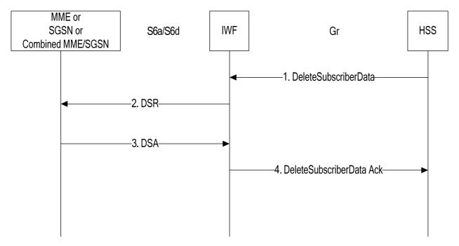
Figure 7.6.1-1: Mapping of Delete Subscriber Data Procedure for scenario with one IWF
