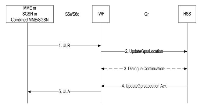
Figure 7.2.1-1: Mapping of Update Location Procedure for scenario with one IWF
