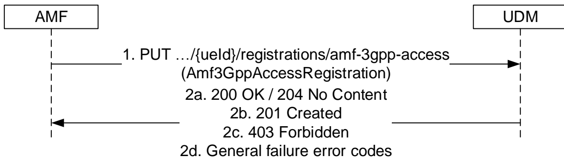
Figure 5.3.2.2-1: AMF registering for 3GPP access
