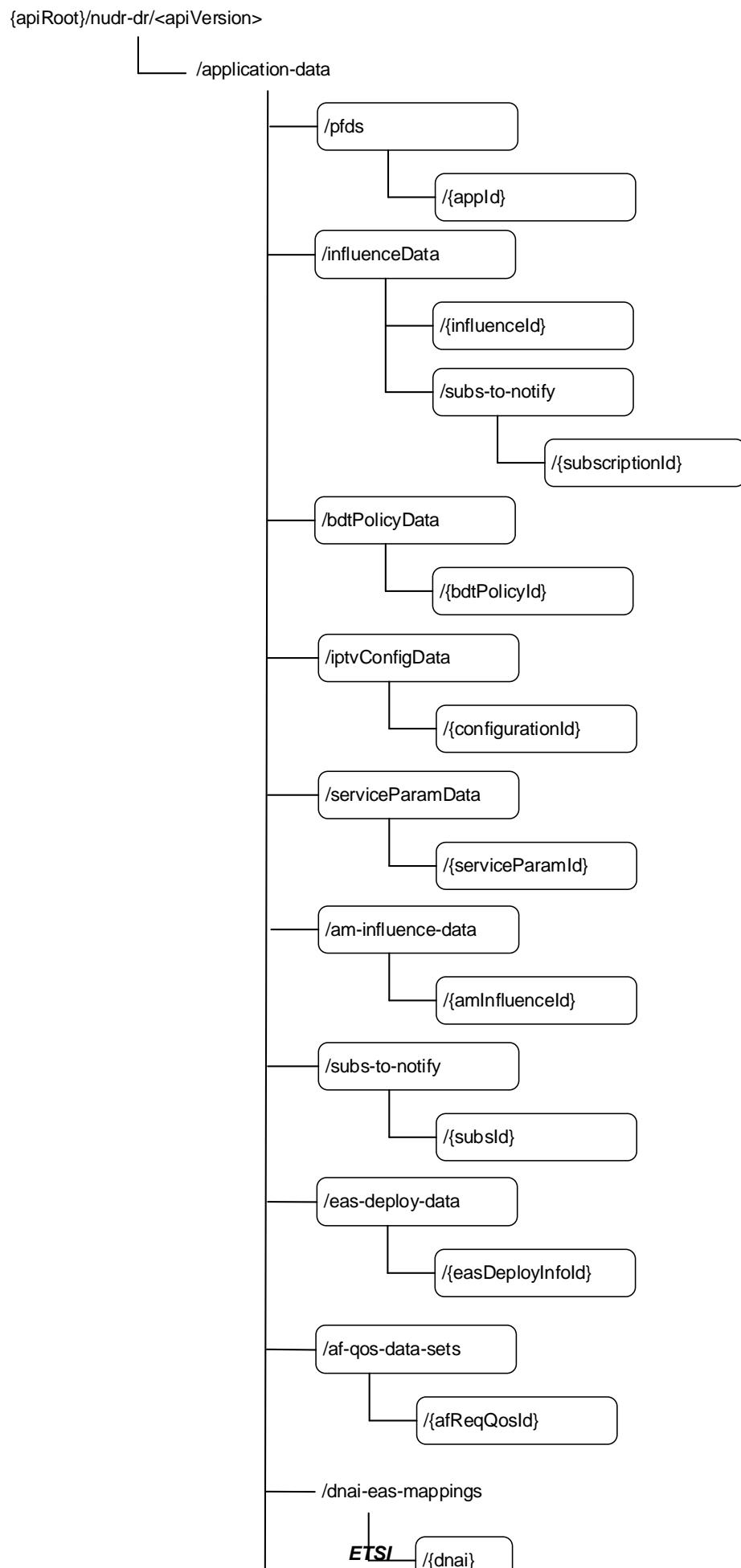
**Figure 6.2.2-1: Resource URI structure of the Nudr\_DataRepository API for application data**
