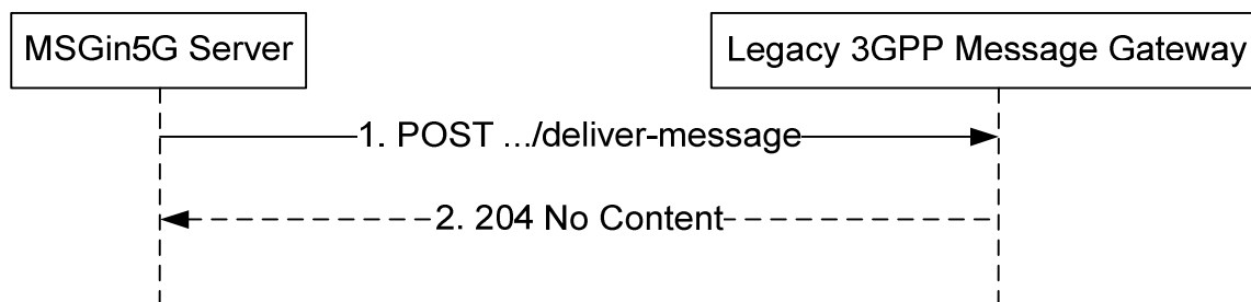
Figure 6.2.2.2-1: Legacy 3GPP Message Gateway Terminating Message Delivery
