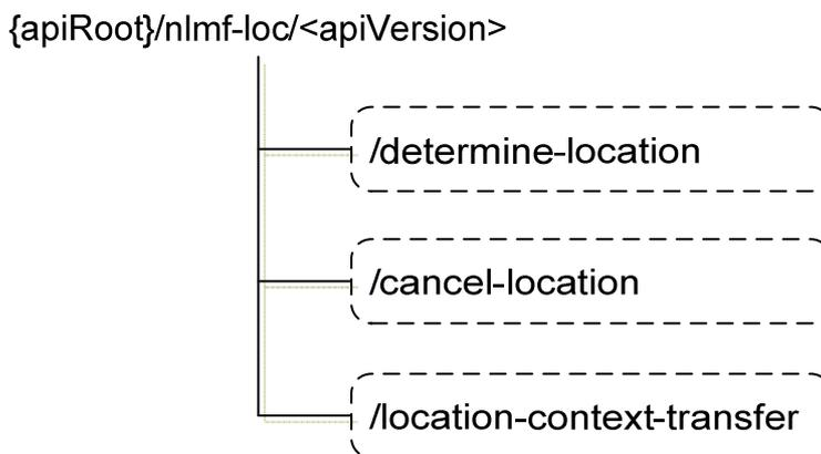
Figure 6.1.3.1-1: Resource URI structure of the Nlmf\_Location API
