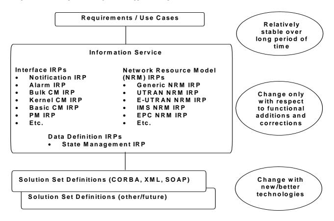
Figure 4.2-1: The IRP 3-level specifications approach combined with the three IRP categories
