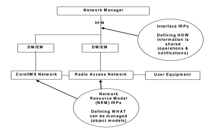
Figure 4.2-2: Relationship Interface IRP vs NRM IRP
