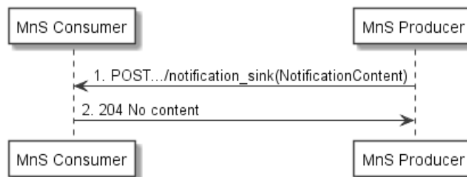
Figure 5.5.4-1: Flow for sending a notification
