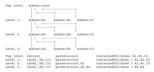
When reading/writing self-contained classes only the last such class instance needs to be specified in the Netconf request as that uniquely identifies the exact instance. The following Netconf request could be used to retrieve all attributes of SubNetwork=root, SubNetwork=A1, SubNetwork=B2, NRFrequency=22
