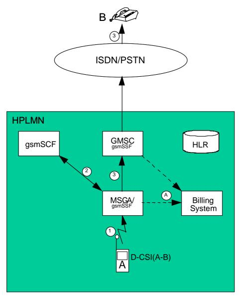
Figure 5.2.1.20: Outgoing call handled by CAMEL with Dialled CSI Trigger
