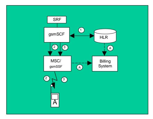
Figure 5.2.1.23: Wake-up call handled by CAMEL CPH
