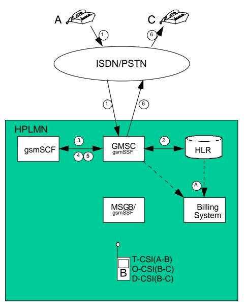
Figure 5.2.1.21: Incoming call handled by CAMEL with redirection decided and forwarding leg handled by CAMEL with Dialled CSI Trigger
