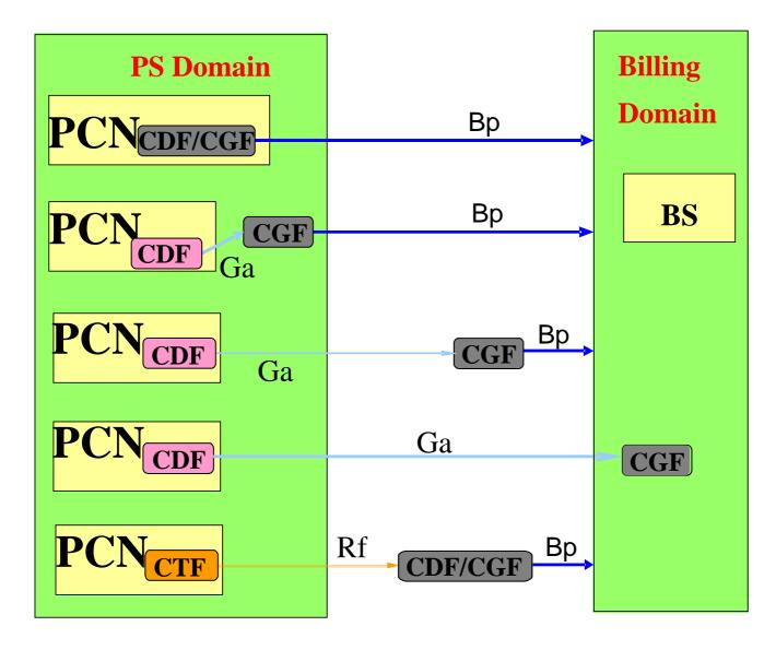
Figure 4.2-1: PS domain offline charging architecture
