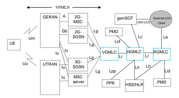
Figure 4.1.1: LCS logical architecture with inter-GMLC [Lr] interface
