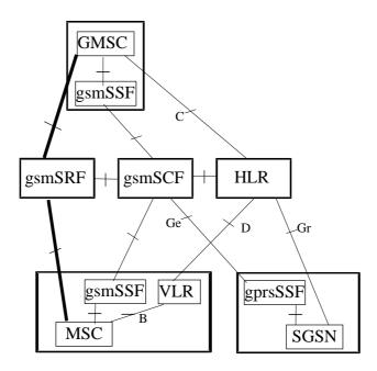
NOTE: The bold lines are used for interfaces supporting user data only, the dashed lines are used for interfaces supporting signalling only.
