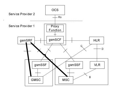
Figure 4.3.1: VCS from a Proxy Function online charging architecture
