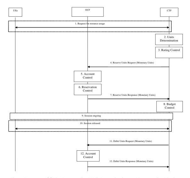
Figure 5.2.2.3.3.1: SCUR - Decentralized Unit Determination and Decentralized Rating
