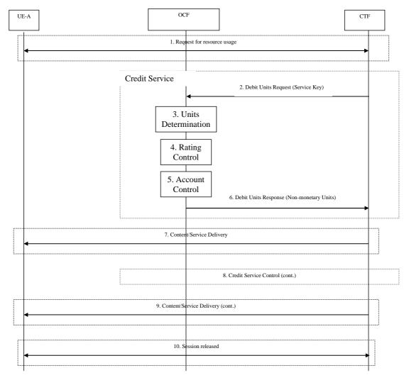
Figure 5.2.2.1.2.1: IEC - Centralized Rating and Centralized Unit Determination
