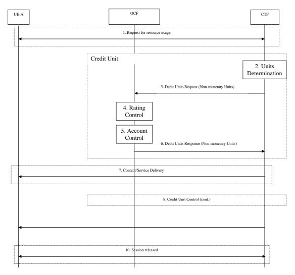
Figure 5.2.2.1.1.1: IEC - Centralized Rating and Decentralized Unit Determination
