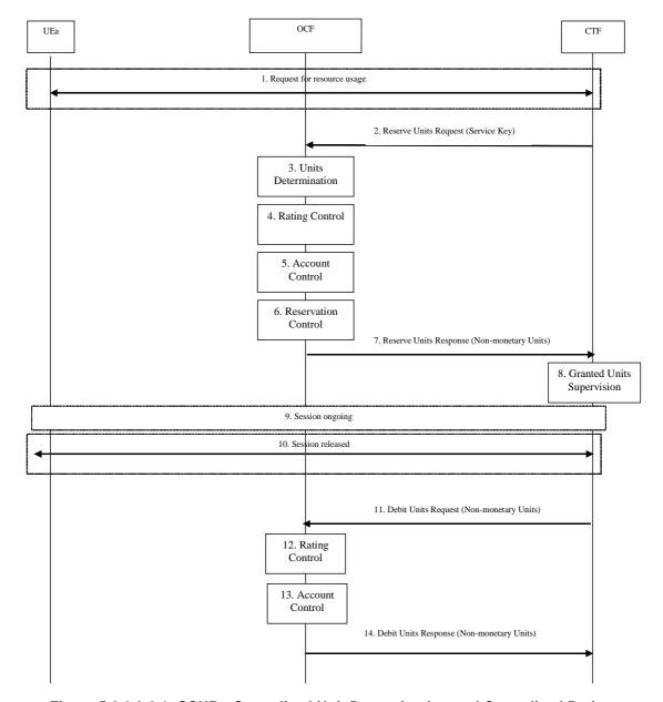
Figure 5.2.2.3.2.1: SCUR - Centralized Unit Determination and Centralized Rating
