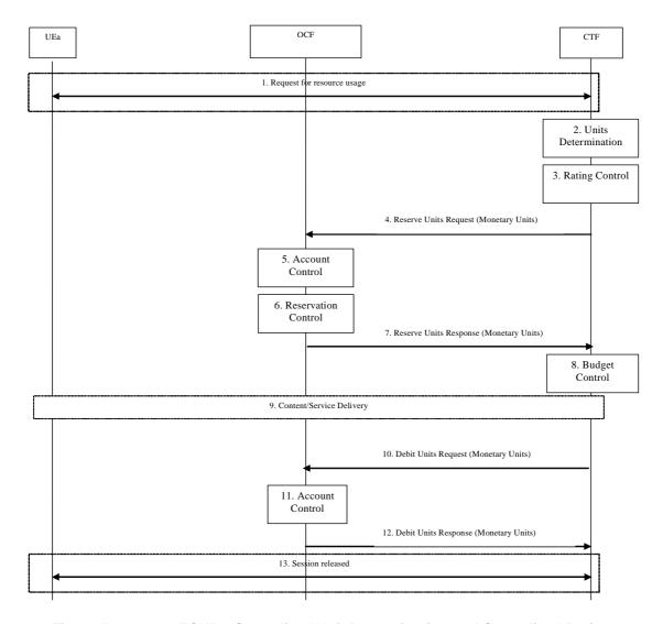
Figure 5.2.2.3.1: ECUR - Centralized Unit Determination and Centralized Rating
