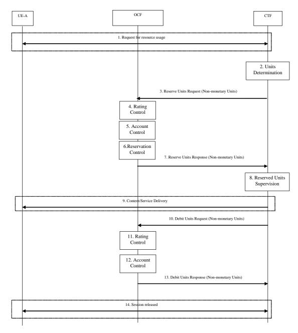
Figure 5.2.2.1.1: ECUR - Decentralized Unit Determination and Centralized Rating
