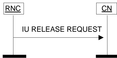
Figure: Iu Release Request procedure. Successful operation
