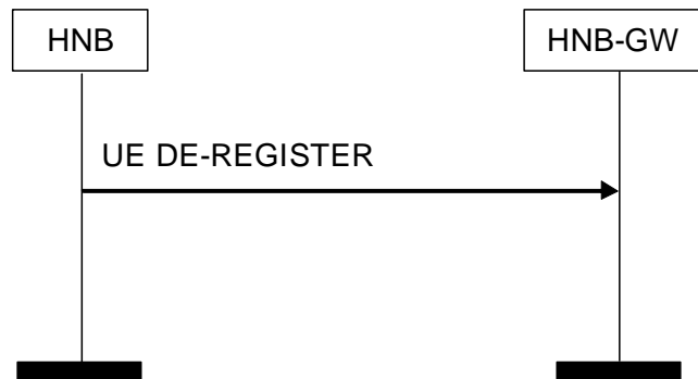
Figure 3 UE De-Register Procedure: HNB Originated Successful Operation
