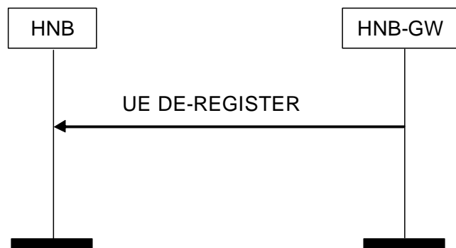
Figure 4 UE De-Register Procedure: HNB-GW Originated Successful Operation
