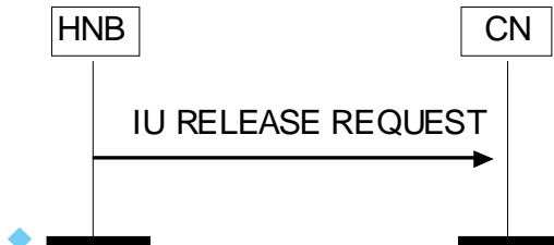
Figure 12 Iu Release Request procedure. Successful operation
