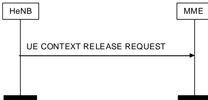
Figure 7 UE Context Release Request procedure. Successful operation
