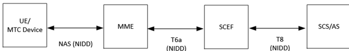
Figure 7.10-1: EPS Architecture for NIDD using SCEF
