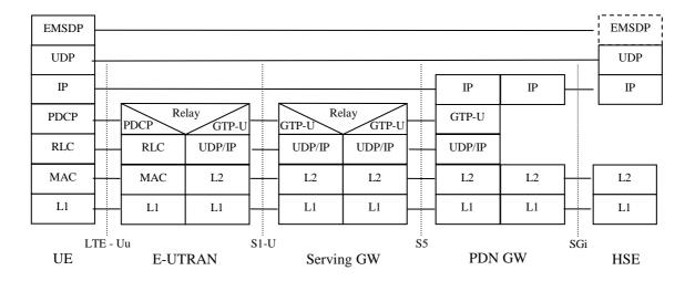
Figure 6.2.1-3: IP data stack for the EMSDP transfers
