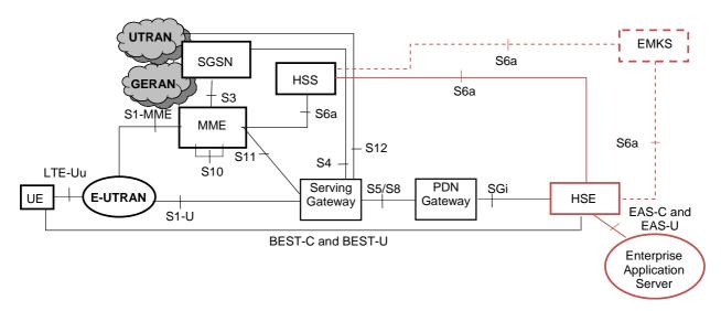
Figure 4.2.1-1: The architecture of the extended user plane protection service
