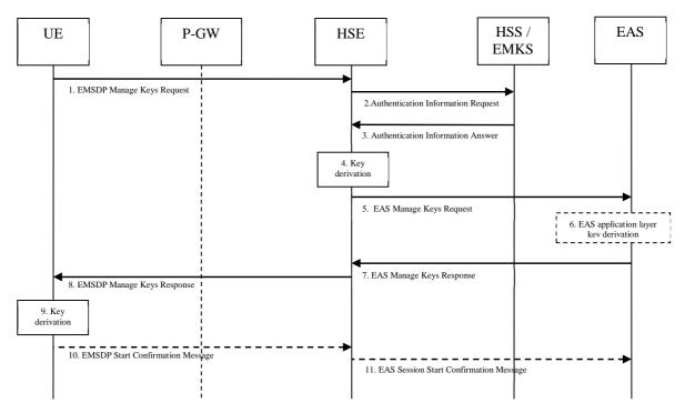
Figure 6.2.7.2-2: BEST Procedure for Key Refresh using EMSDP
