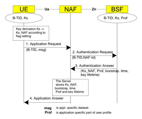
Figure I.4: The bootstrapping usage procedure
