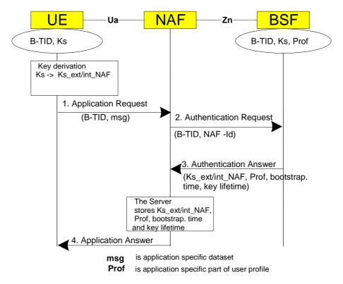
Figure 5.3: The bootstrapping usage procedure with UICC-based enhancements
