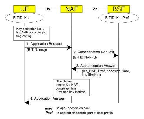
Figure I.4: The bootstrapping usage procedure
