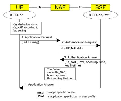
Figure 4.4: The bootstrapping usage procedure
