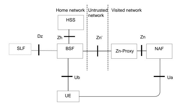
NOTE: The Zn' reference point is distinguished from the Zn reference point in that it is used between operators.
