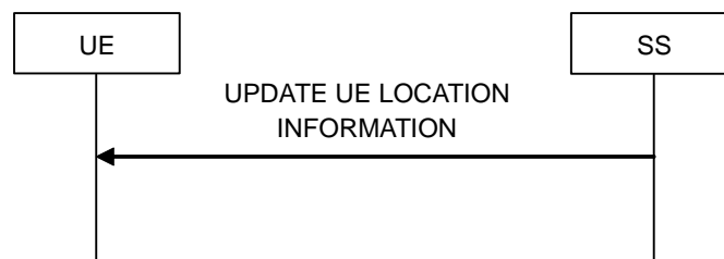
Figure 5.4.2-1: Update UE Location Information procedure
