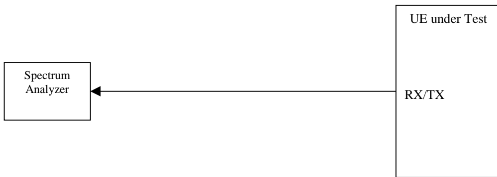
Figure A.7: Connection for RX Test with both Interference and additional CW
