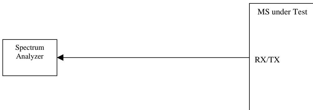
Figure A.8: Connection for Spurious Emission Test
