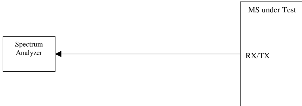
Figure A.8: Connection for Spurious Emission Test
