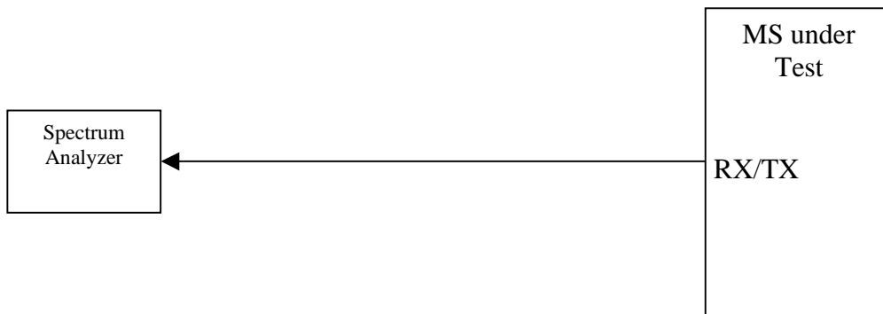
Figure A.8: Connection for Spurious Emission Test
