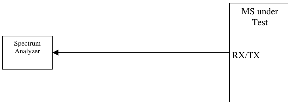
Figure A.8: Connection for Spurious Emission Test
