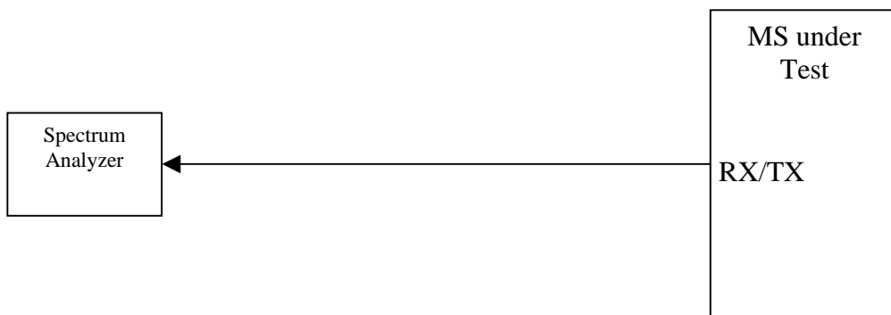
Figure A.8: Connection for Spurious Emission Test
