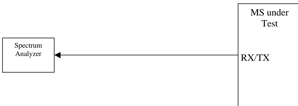
Figure A.8: Connection for Spurious Emission Test
