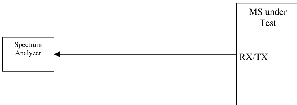
Figure A.8: Connection for Spurious Emission Test
