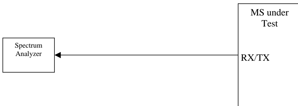
Figure A.8: Connection for Spurious Emission Test
