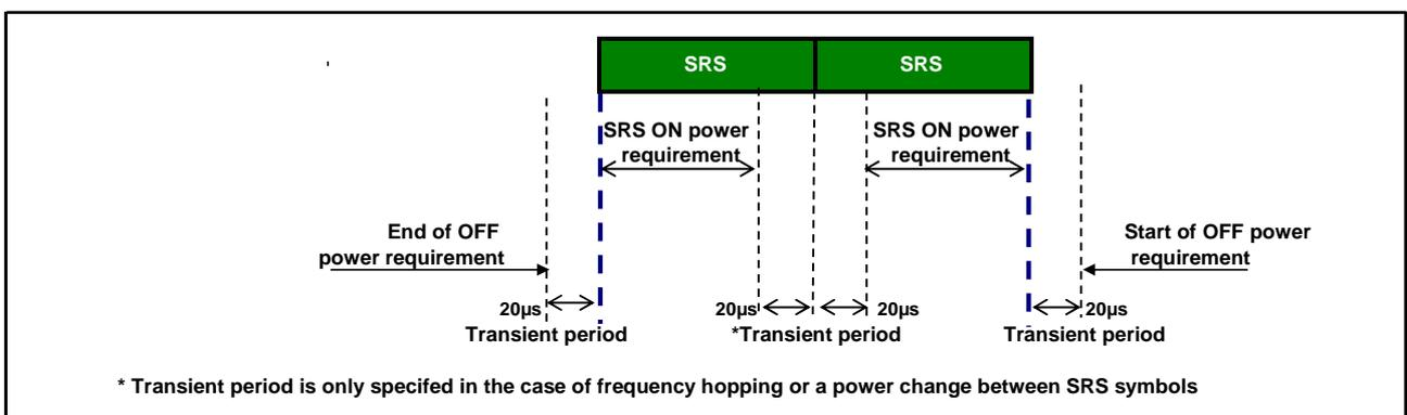
\* Transient period is only specified in the case of frequency hopping or a power change between SRS symbols
