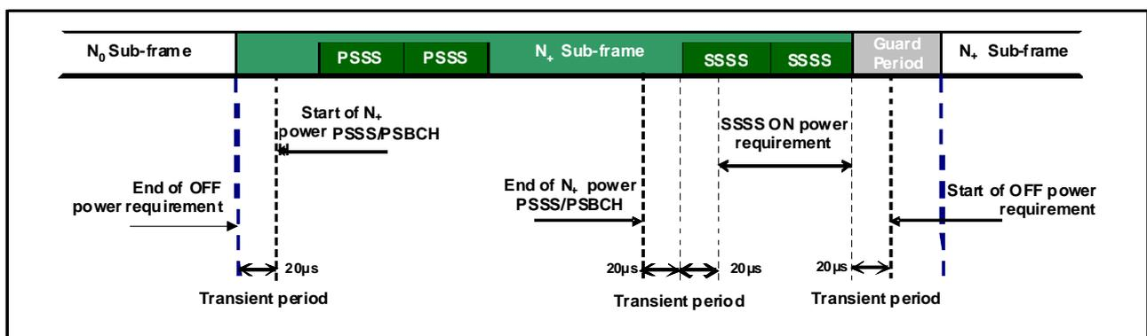
**Figure 6.3.4G.1-1: PSSS/SSSS/PSBCH time mask for normal CP transmission for V2X Service**
