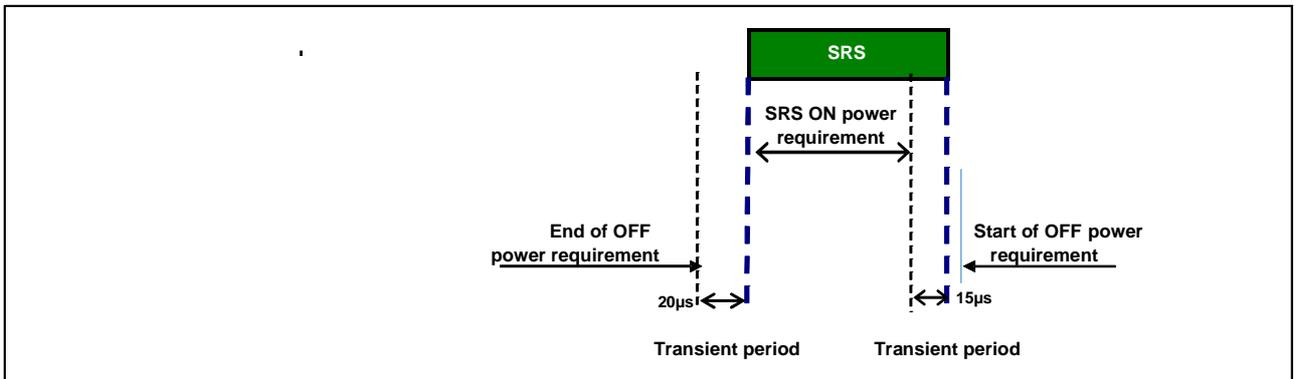
Figure 6.3.4.2.2-1A: Single SRS time mask for Frame Structure Type 3
