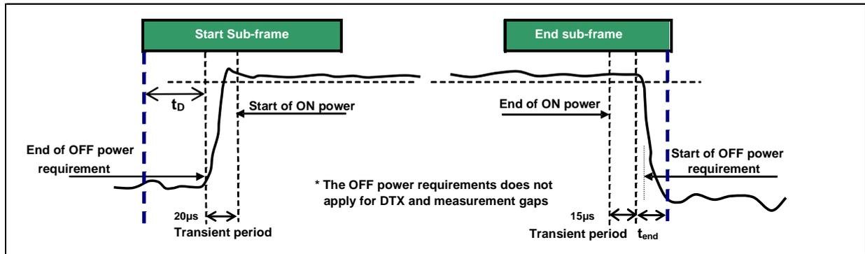
Figure 6.3.4.1-1A: General ON/OFF time mask for Frame Structure Type 3
