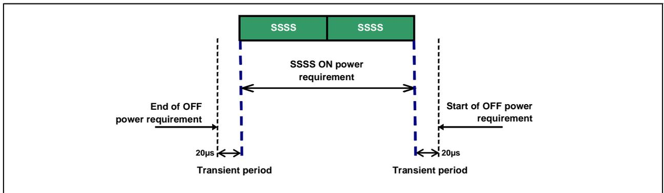
Figure 6.3.4D.2-3: SSSS time mask (when not time-multiplexed with PSBCH)
