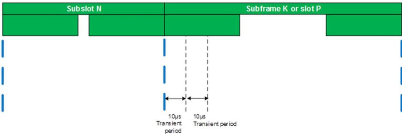
Figure 6.3.4.9-1: subslot TTI and subframe TTI boundary
