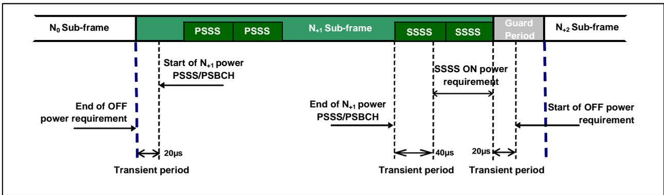
Figure 6.3.4D.3-1: PSSS/SSSS/PBCH time mask for normal CP transmission
