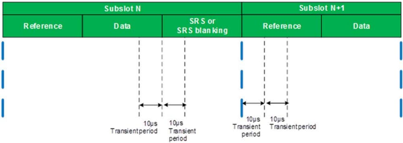
Figure 6.3.4.6-4: subslot PUSCH/SRS time mask when there is a data symbol before SRS (or SRS blanking) and Reference symbol after
