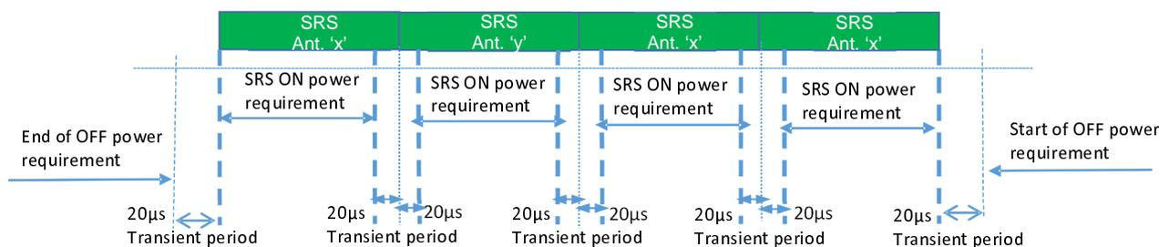
**Figure 6.3.4.2.2-5: Time mask for SRS antenna switching**
