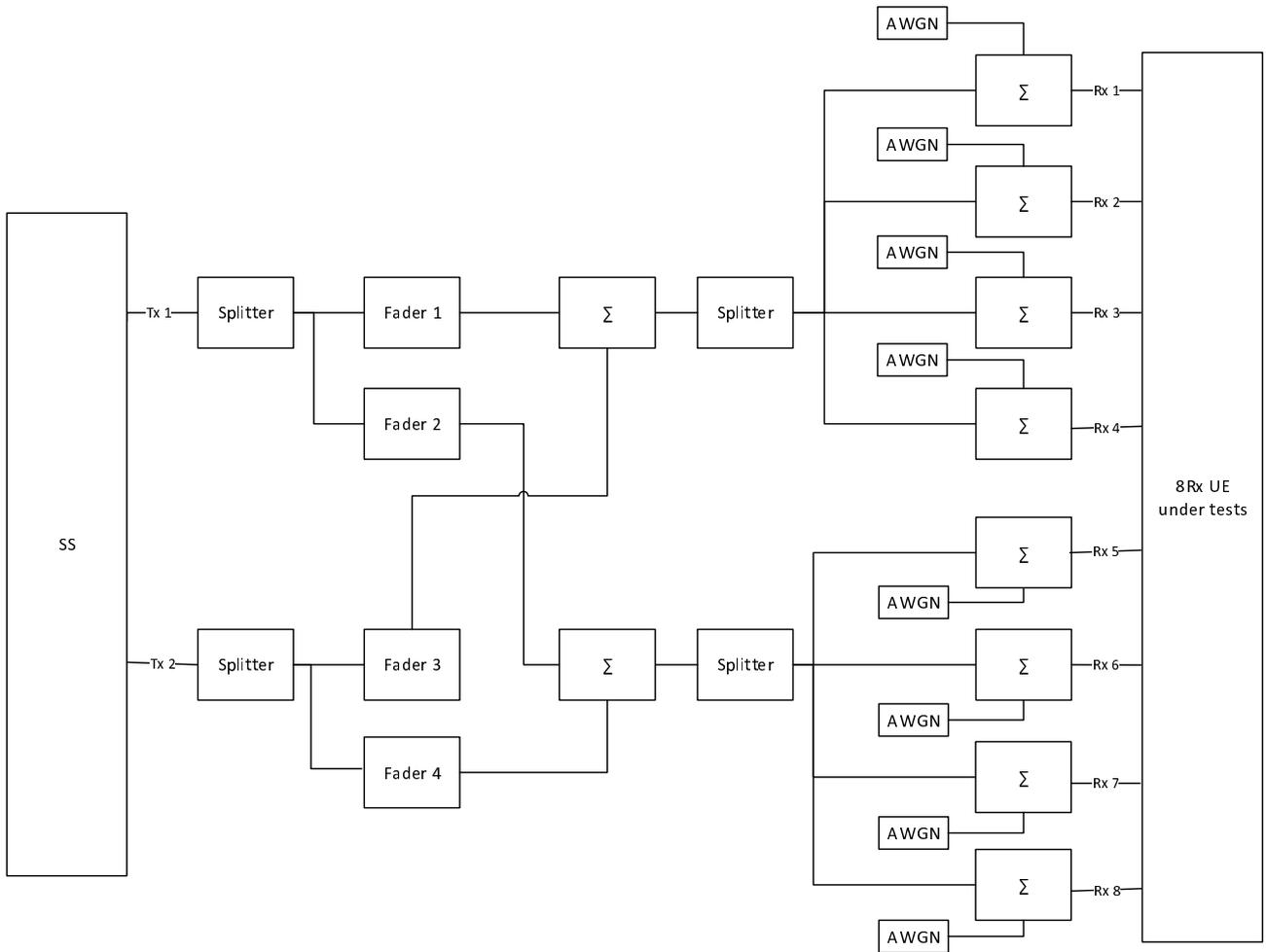
**Figure 8.1.2.12.1-1: Antenna connection example for 2Rx tests with antenna configuration as 2x2 without interference (informative)**
