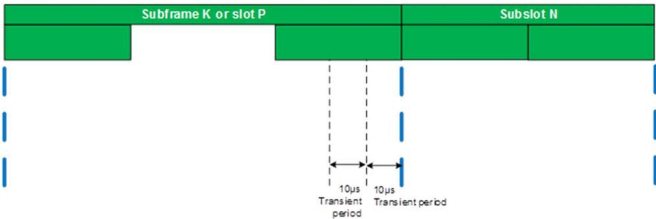
**Figure 6.3.4.10-3: subframe TTI and subslot TTI boundary**
