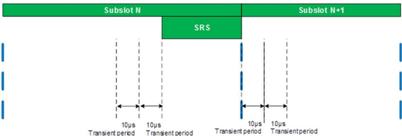
Figure 6.3.4.6-7: subslot PUSCH/SRS time mask when there is a no symbol before and after SRS
