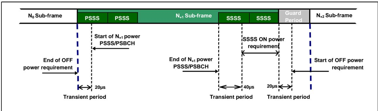
Figure 6.3.4D.3-2: PSSS/SSSS/PBCH time mask for extended CP transmission
