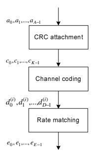
Figure 5.3.1-1: Transport channel processing for BCH.
