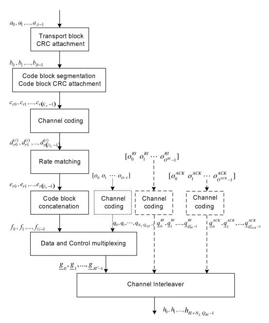
Figure 5.2.2-1: Transport block processing for UL-SCH.
