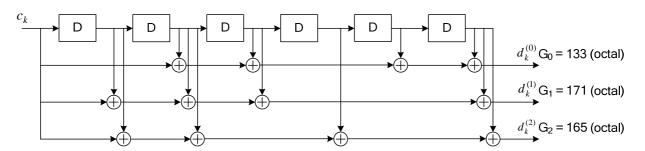
Figure 5.1.3-1: Rate 1/3 tail biting convolutional encoder.
