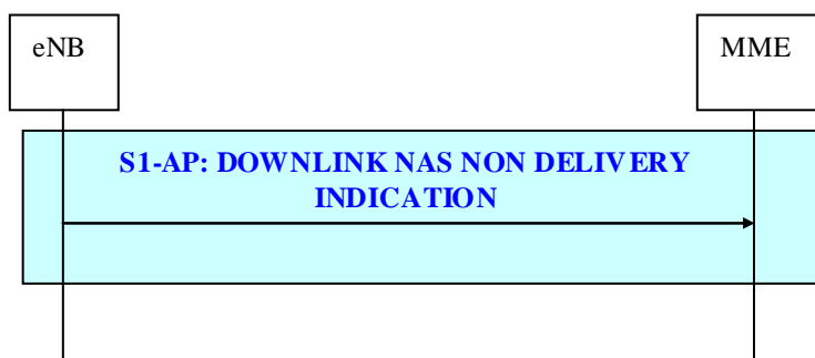
Figure 19.2.2.6-4: Downlink NAS Non Delivery Indication procedure
