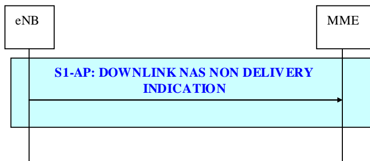
Figure 19.2.2.6-4: Downlink NAS Non Delivery Indication procedure
