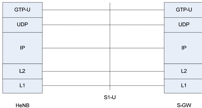
Figure 4.6.3.1-1: User plane for S1-U interface for HeNB without HeNB GW
