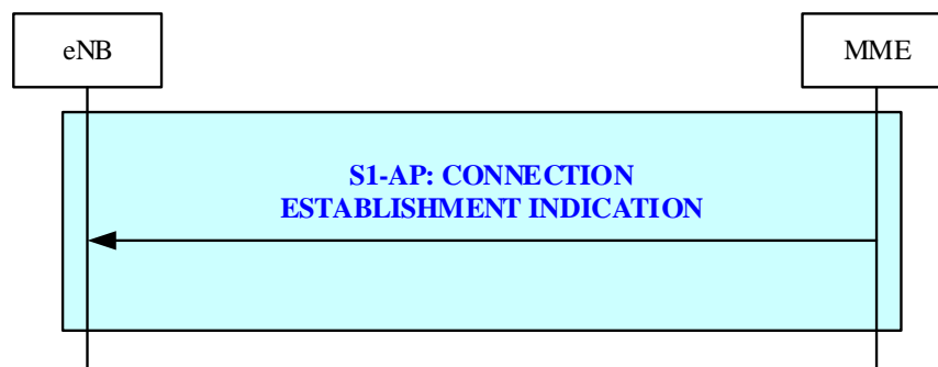
Figure 19.2.2.25-1: Connection Establishment Indication procedure
