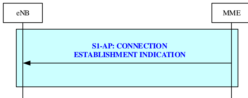
Figure 19.2.2.25-1: Connection Establishment Indication procedure
