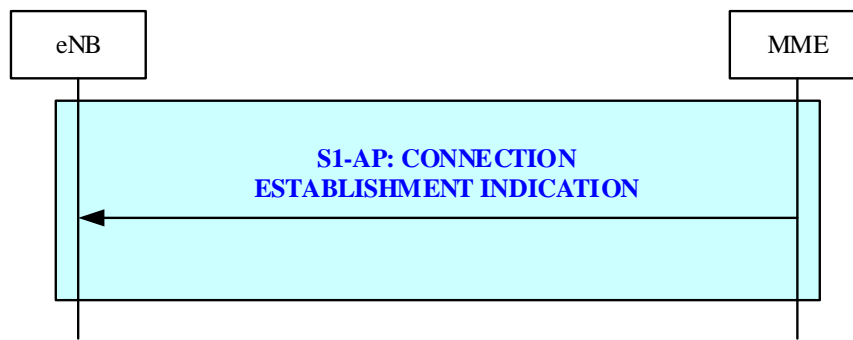
Figure 19.2.25-1: Connection Establishment Indication procedure
