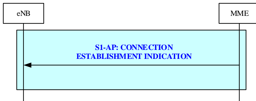
Figure 19.2.25-1: Connection Establishment Indication procedure
