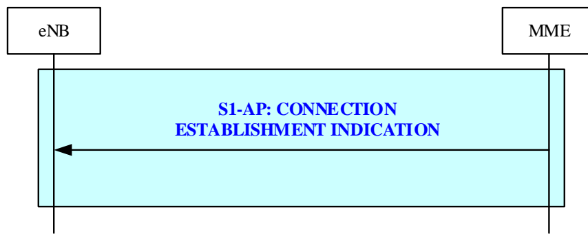
Figure 19.2.25-1: Connection Establishment Indication procedure
