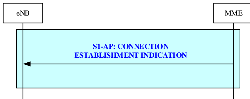
Figure 19.2.25-1: Connection Establishment Indication procedure
