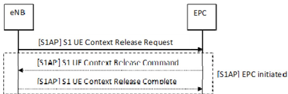
Figure 19.2.2.2.2-1: S1 UE Context Release Request procedure (eNB triggered) and subsequent S1 UE Context Release procedure (EPC triggered)
