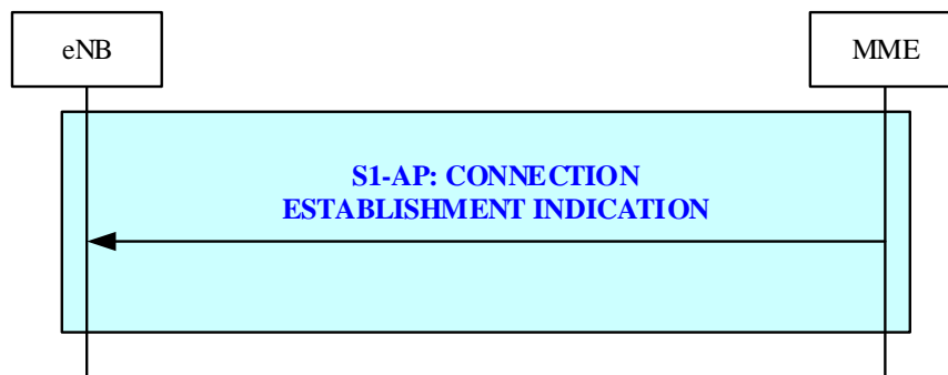
Figure 19.2.25-1: Connection Establishment Indication procedure
