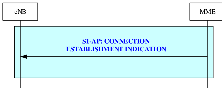
Figure 19.2.25-1: Connection Establishment Indication procedure
