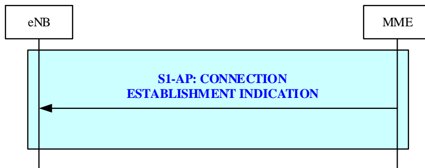
Figure 19.2.25-1: Connection Establishment Indication procedure
