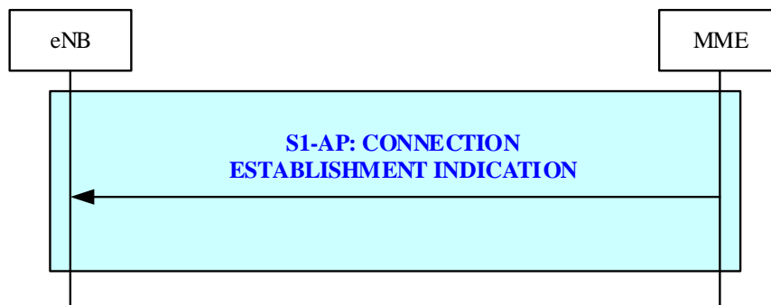
Figure 19.2.25-1: Connection Establishment Indication procedure
