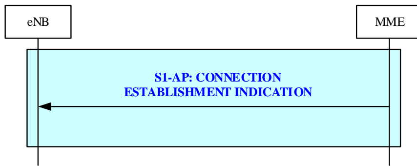
Figure 19.2.25-1: Connection Establishment Indication procedure
