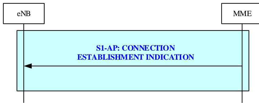
Figure 19.2.25-1: Connection Establishment Indication procedure
