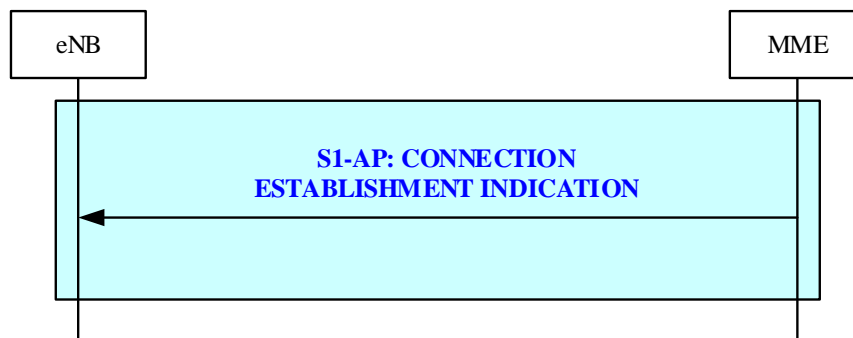
Figure 19.2.25-1: Connection Establishment Indication procedure
